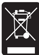
Fig. 1.4: Product labeling in accordance with EN 50419
