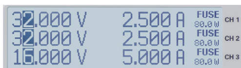
Fig. 5.1: 1-V position for all three channels (R&S®HMP2030)
