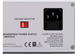
Fig. 1.1: Voltage selector for the R&S®HMP2030
